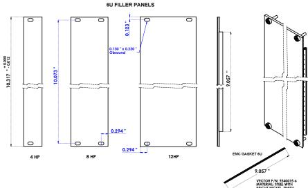
Each Filler Panel Kit Includes 4,8 or 12HP EMC panel with EMC gasket
